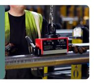
Zero running costs permanent magnetic technology does not require a sustained power source
